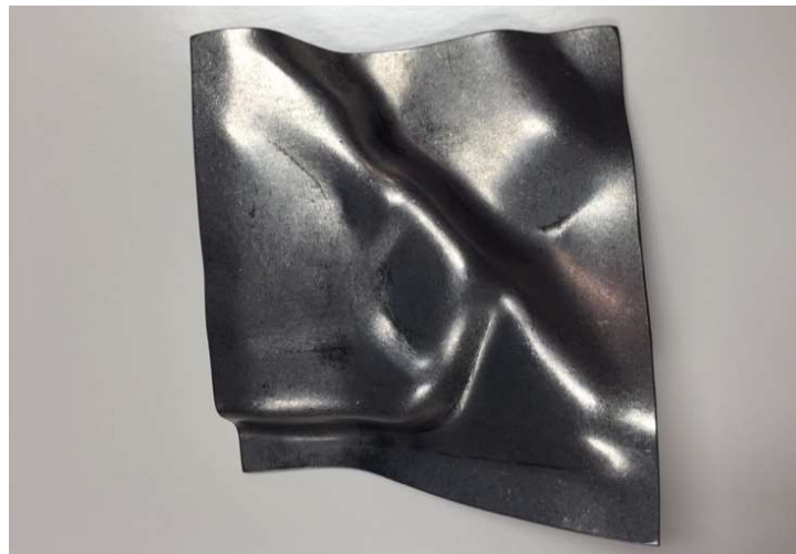
Fig 9: Flash® 1800 (260ksi) prototype 2mm thick x 125mm x 125mm stamping to 2(r/t) bend radii
