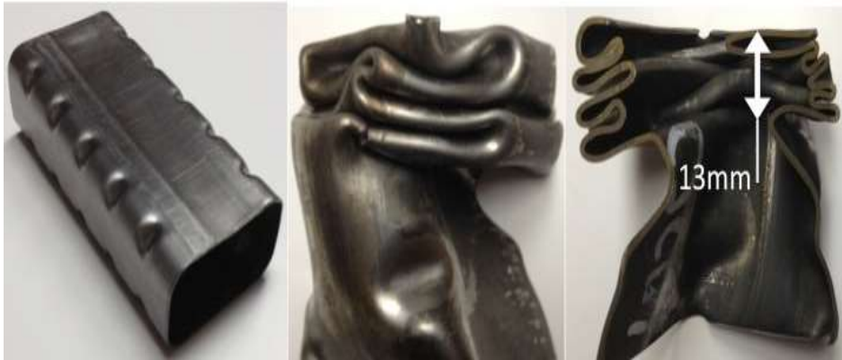
Figure 4 shows a research project for an automotive “crush can” made of Flash® 1500 (225ksi).
